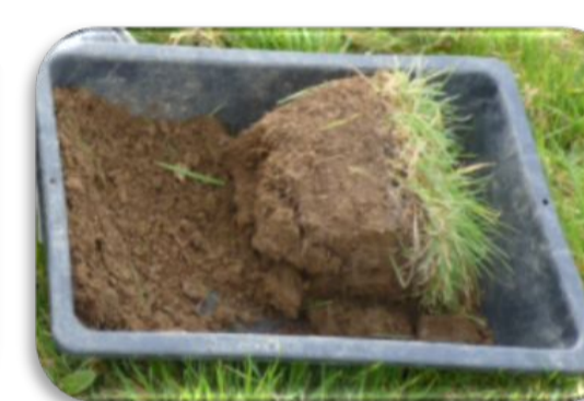
Extraction of soil blocks
